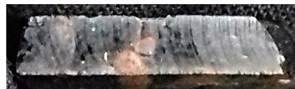
Curved striations from grinding the edge flat - this is the edge closest to the scale at the bottom of the adjacent photograph (south side 2).
